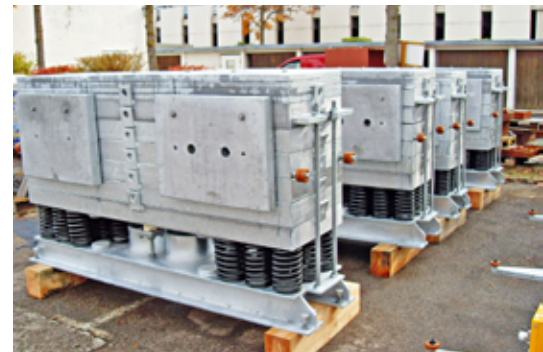
The flame zinced tuned mass damper with a weight of 6,500 kg/unit and a vibration frequency of 1.87 Hz prior to installation at the pedestrian bridge leading to the Auto City of Wolfsburg.
