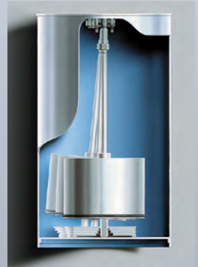
Active principle of a MAURER friction pendulum damper as a multi-disc system with pendulum mass to dampen wind-induced vibrations of steel stacks
