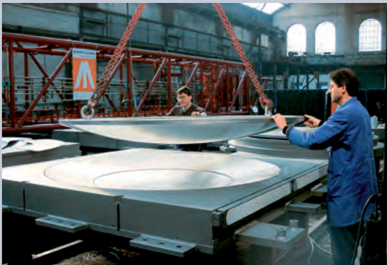
Assembly of a spherical bearing for loads up to 131,000 kN in the historical hall 1 of Maurer Söhne
