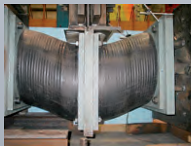
Dynamic shear test at self-produced and especially composed MAURER elastomeric isolators, produced for an uranium enrichment plant in France
