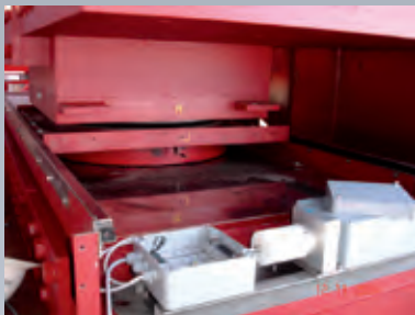
Monitoring system for permanent online control of bearing deformations at the Tejo Bridge "25th April" in Lisbon, Portugal
